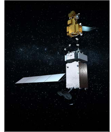
Restore-L (silver), a spacecraft capable of robotically repairing satellites (gold) in orbit. Courtesy NASA
